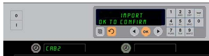
Cabinet configuration file names on the flash drive are visible on the cabinet (top) when importing a configuration. A configuration is selected by pressing the adjacent timer button. That file name appears in the top left position (lower illustration). All timer buttons are extinguished and all other row positions displays are blank.
